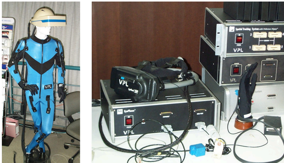
FIGURE 1.9: VPL's products. Left: Datasuit. Right: EyePhone & Dataglove. (Sources: Left: [Pap99a], Right: [Pap99b])
