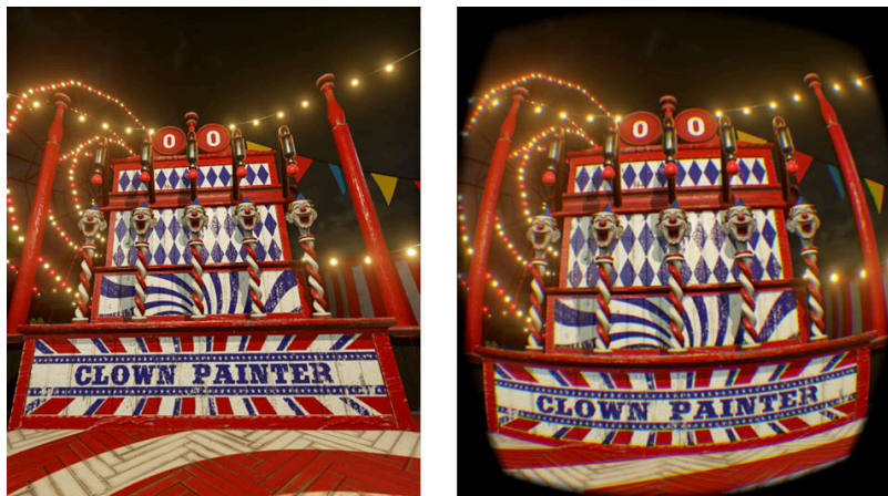
FIGURE 2.27: Effects of lens distortion on a rectilinear image. (Sources: [Liu17])
