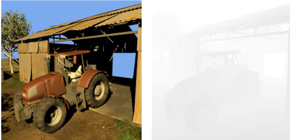
FIGURE 2.24: Depth buffer. Depth buffer values (0 to 1), determine the depth of the pixel. Darker pixels typically represent geometry that is closer. (Image rendered using XEngine [PV13])
